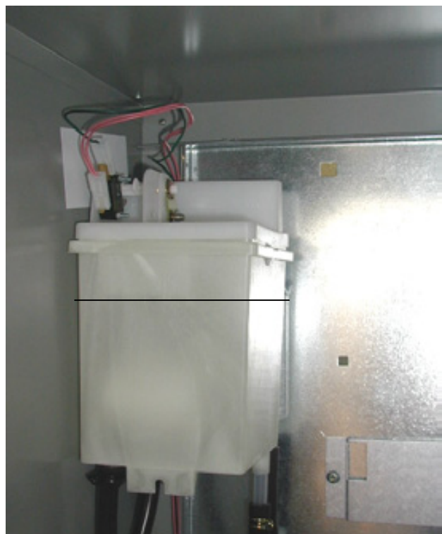
Air-break: application on the Spazio
